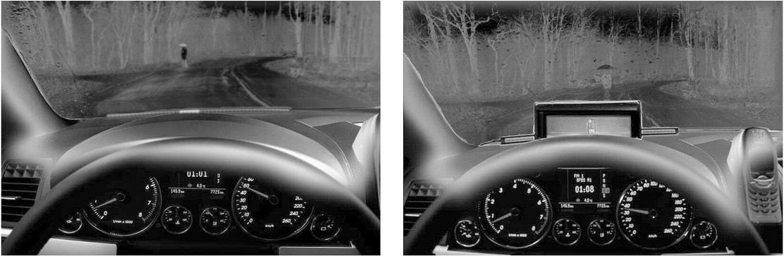
Figure 2. Examples for two different display types: APR-LED (left) and APR-MHU (right). (See Table 1 for explanations of abbreviations.)
