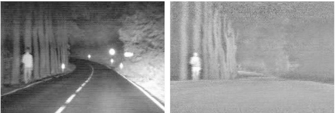
Figure 1. Sensor images: near infrared (left) and far infrared (right).
